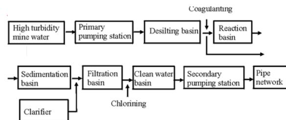
Figure 3. Purification process of high-turbidity water.
