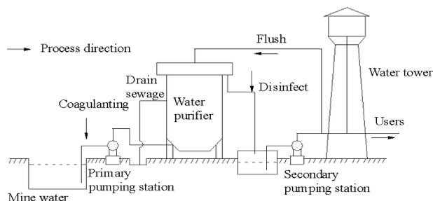
Figure 5. Purification process of the integrative water purifier.
