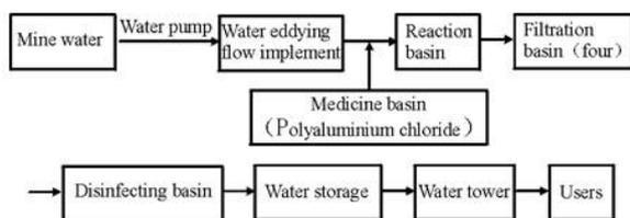
Figure 4. Purification process of the mine water in Wannian Coal Mine.
