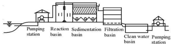
Figure 1. Schematic diagram showing the purification.
