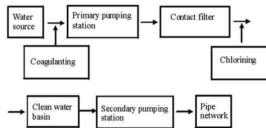
Figure 2. Purification process of low-turbidity water.
